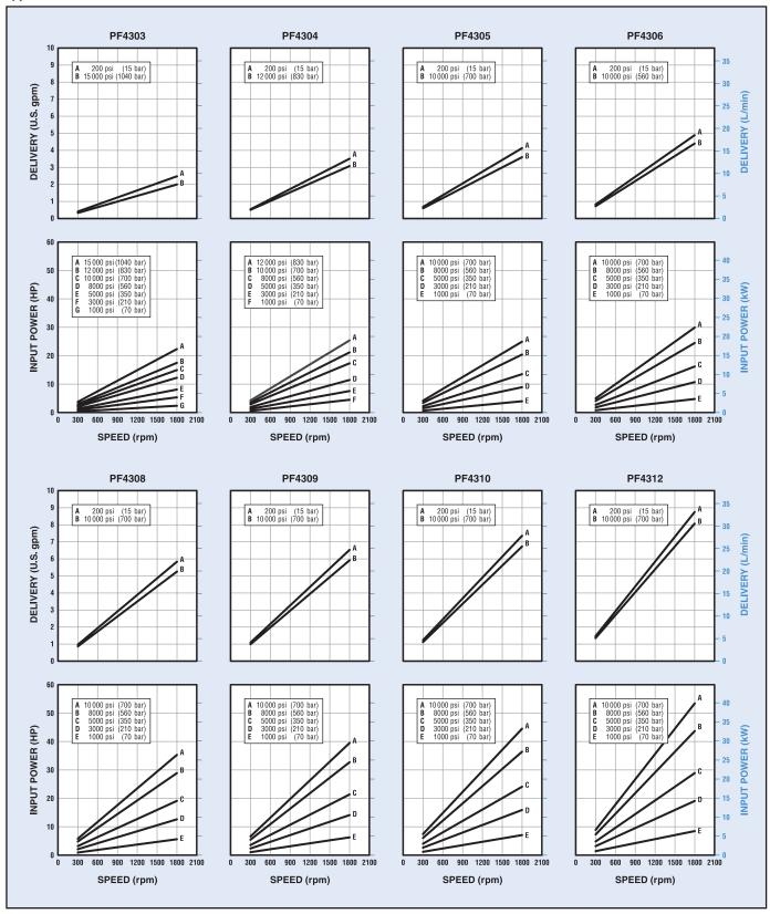
Typical performance curves are based on 33 SUS (1,9 cSt) water glycol fluid with pressurized inlet where required. Refer to the "Minimum Inlet Pressure" table on page 2.
